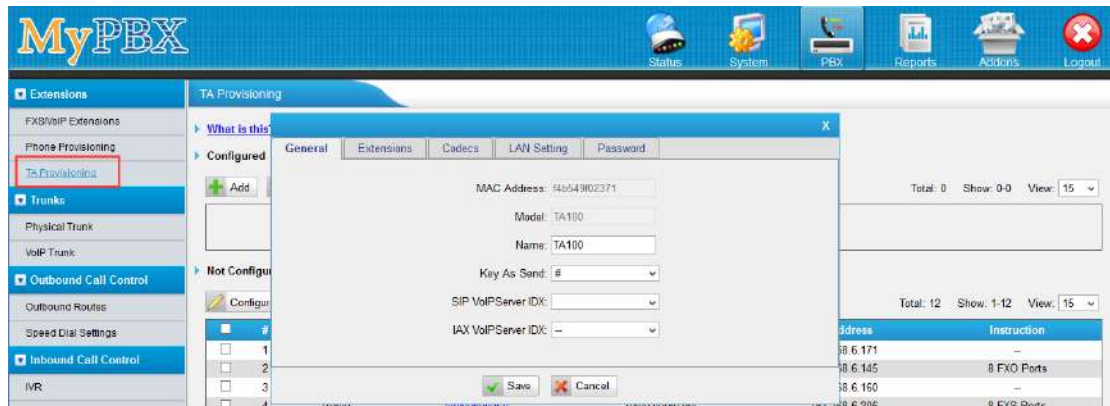
Figure 11-4 MyPBX TA Provisioning
